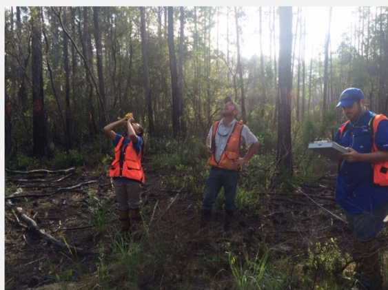
Andraya uses a clinometer to measure tree heights.
